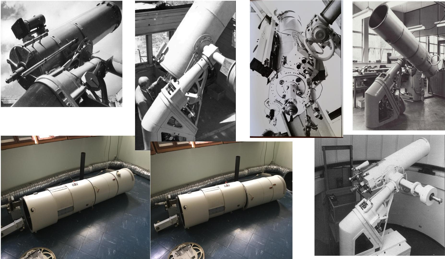
**Plate 10** Catts/University telescope. Clockwise from top left: The original configuration with 51 cm OTA (Credit: Orchiston). The Catts at MSO (Credit: MSO). In Cassegrain mode with a rectangular spectroscope at the Perth Observatory (Credit: Perth Observatory). The renovations in UWA Physics workshop (Credit: UWA). The re-renovated Universitytelescope as a 406 mm (Credit: Perth Observatory). The 2017 pices: Cassegrain layout and Newtonian layout (Credit: Perth Observatory).
