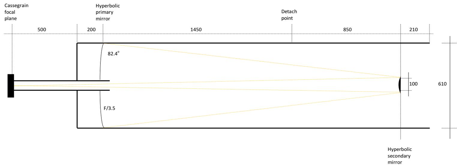
**Plate 15** Schematic light path of the Boller & Chivens Perth Lowell F/75 telescope. All measurements are approximate (Credit: Hunt)
