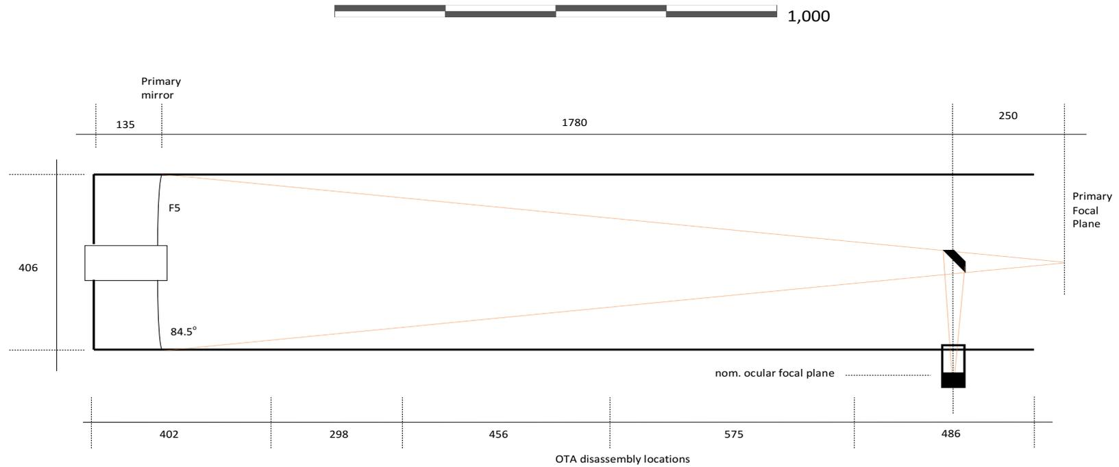
**Plate 12** Schematic light path of the Catts/University Newtonian telescope. All measurements are approximate (Credit: Hunt)
