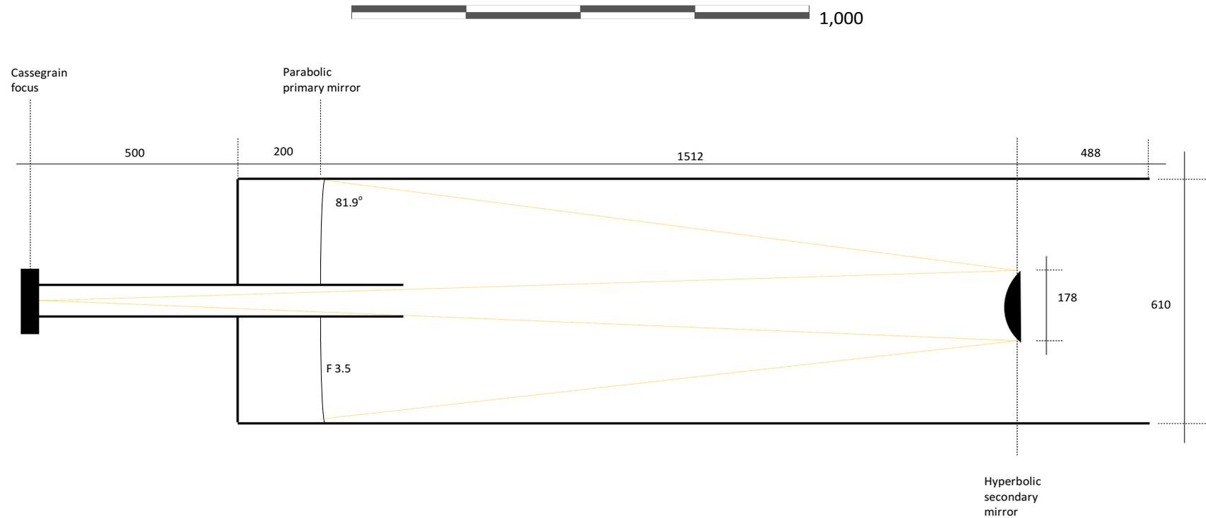
**Plate 14** Schematic light path of the Boller & Chivens Perth Lowell F/13.5 telescope. All measurements are approximate (Credit: Hunt)
