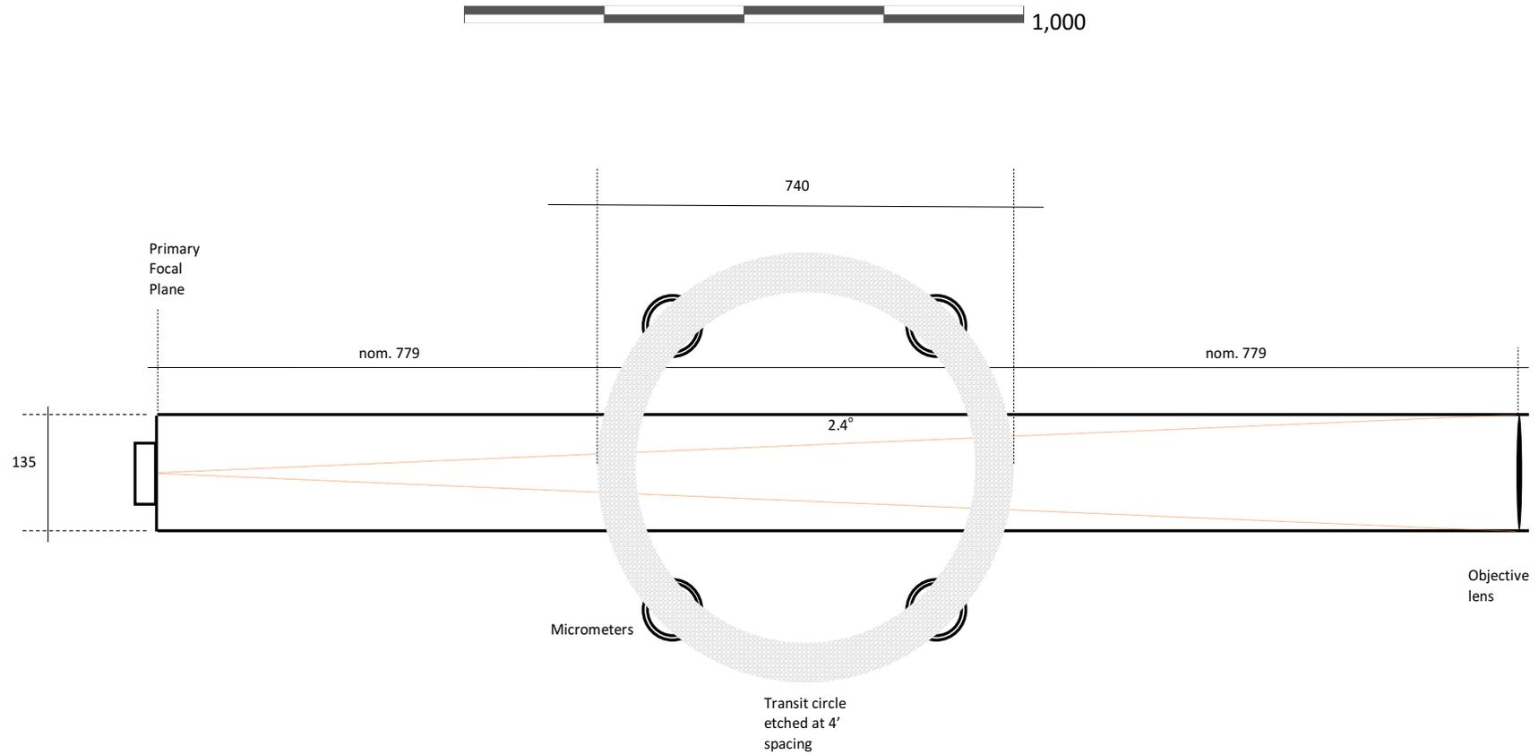
**Plate 7** Schematic light path of the Repsold Meridian Transit Circle. All measurements are approximate (Credit: Hunt)
