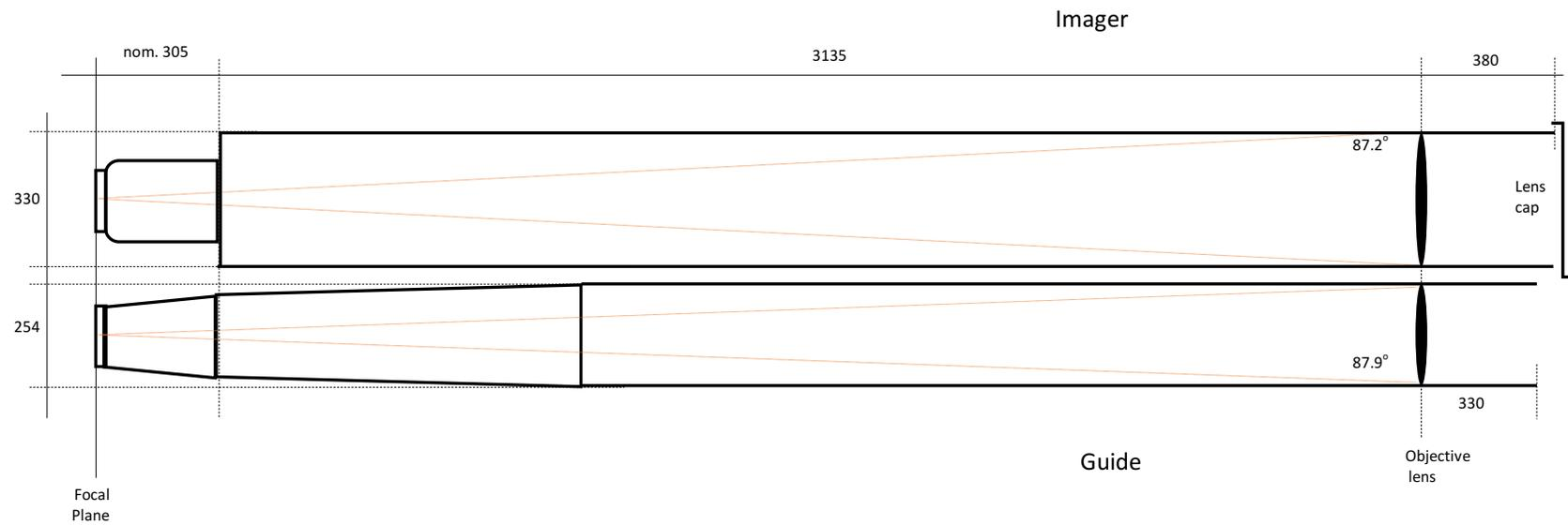
**Plate 9** Schematic light path of the Grubb Astrographic telescope. All measurements are approximate (Credit: Hunt)
