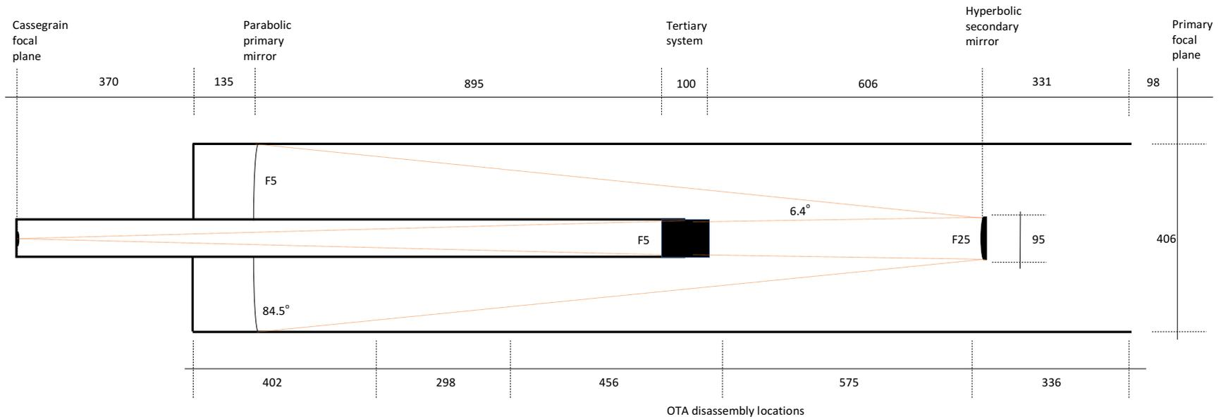
**Plate 11** Schematic light path of the Catts/University Cassegrain telescope. All measurements are approximate (Credit: Hunt)
