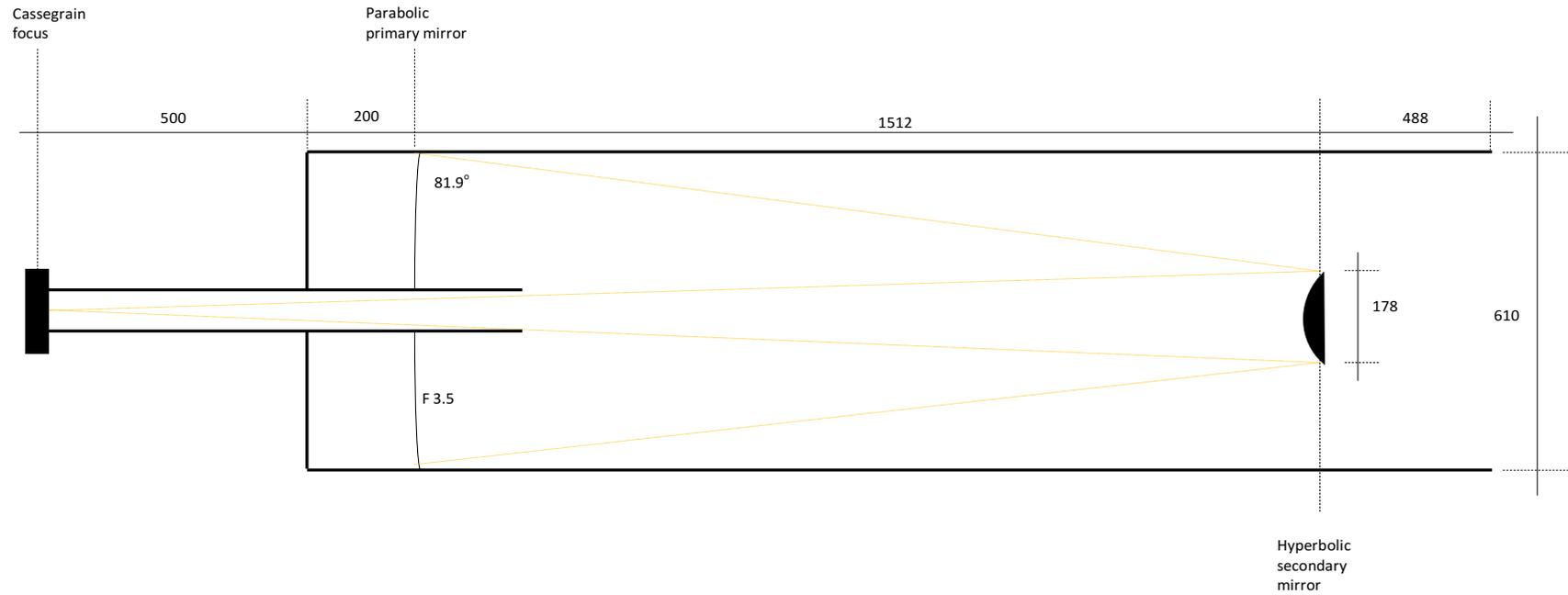
**Plate 14** Schematic light path of the Boller & Chivens Perth Lowell F/13.5 telescope. All measurements are approximate (Credit: Hunt)
